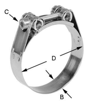
C (screw type) = ISK Diameter D = 73-79Width B = 25
